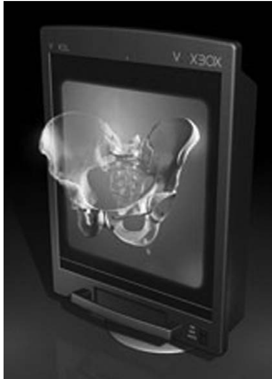
Figure 18-28. Hologram showing a CT image of a pelvic bone in 3D space. A Voxbox® is necessary for visualization (courtesy of Voxel, Inc – Provo – UT, USA).
