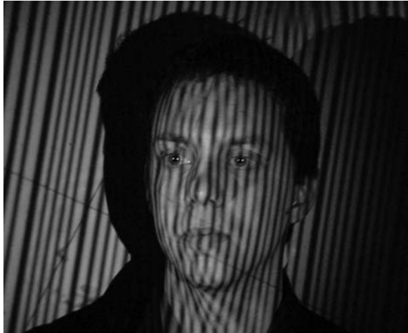
Figure 18-4. Projection of stripe or grid pattern for shape capture using the Face Camera (courtesy of Visual Interfaces, Inc, Pittsburgh, PA)
